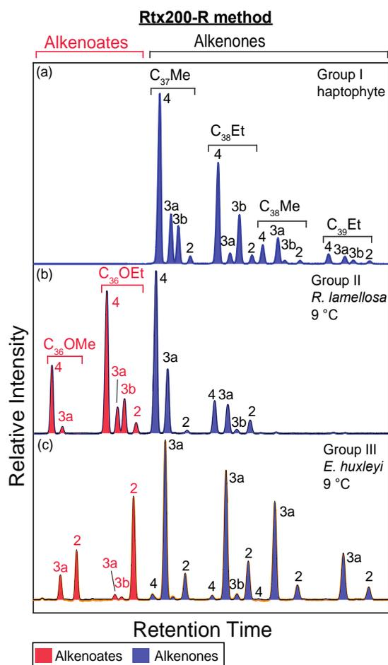
**Figure 1** Gas chromatographic separation of LCAs and LCEs from Group I haptophyte (Greenland sediment, a), Group II haptophyte (*R. lamellosa*, b) and Group III haptophyte (*E. huxleyi*, c) using Restek Rtx-200 column. LCE peaks are filled in red and LCAs in blue. The double bond numbers of LCAs/LCEs are labeled on top of the peaks.
