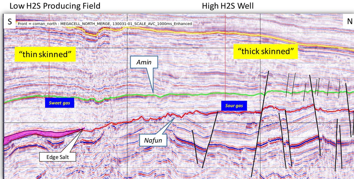
**Figure 1** Cross section between through the high H<sub>2</sub>S structure and the low H<sub>2</sub>S producing field.
