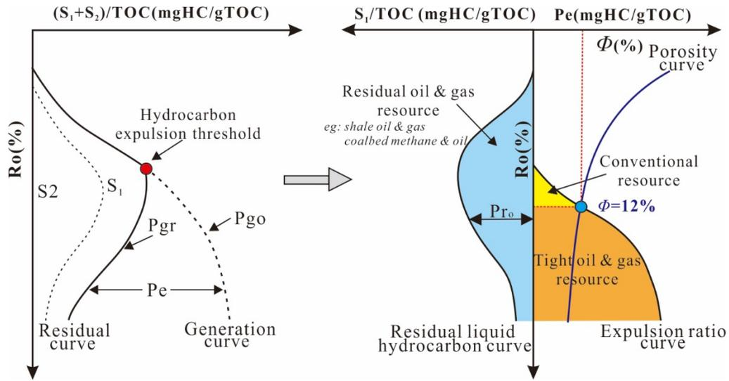
**Figure 1.** Operational model for the qualification of hydrocarbon generation, expulsion and retention
