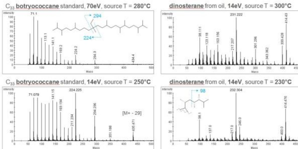
**Figure 1** Examples of mass spectra showing the difference between normal and low-*eV* ionisation and the effect of source temperature.
