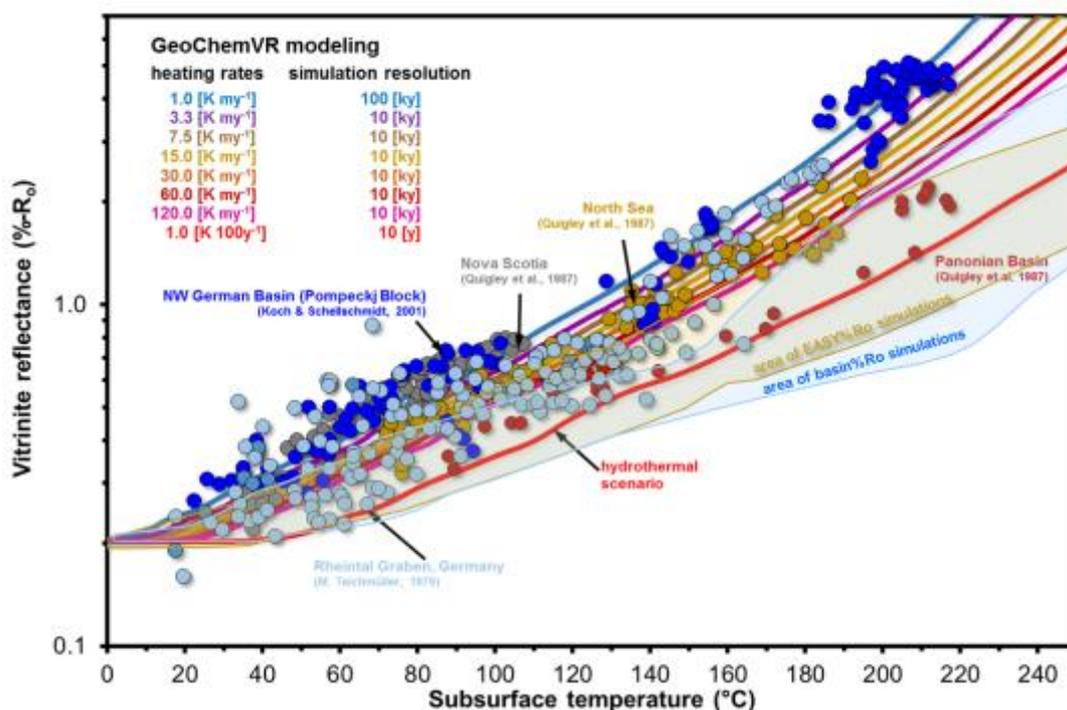
**Figure 1** Simulated vitrinite reflectance (colored lines) using the GeoChemVR concept at different geological heating rates and adequate time resolution in comparison with observations on subsurface temperature and measured vitrinite reflectance. Areas of EASY%Ro and basin%Ro simulations (heating rates from 1 [K/my] to 1 [K/100y]) are given as brown and blue shaded fields, respectively.
